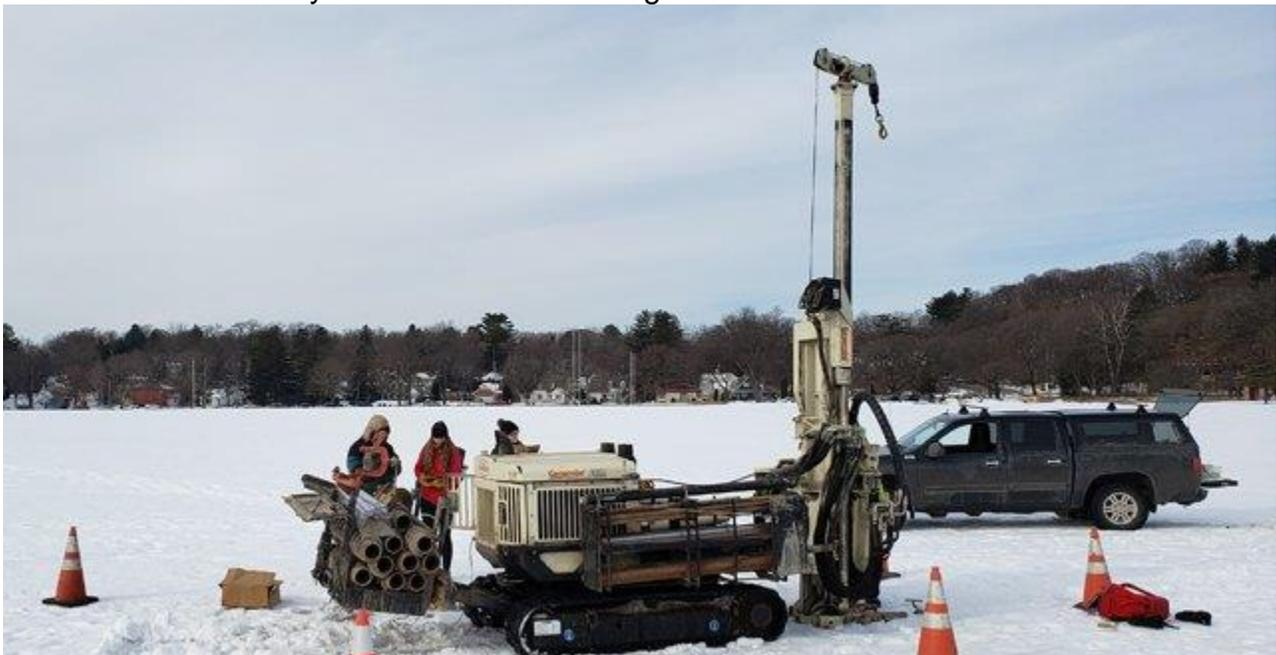
THE GEOPROBE is the piece of equipment, mounted on tracks, that Carson's team uses to take core samples of soils overlaying bedrock. These core samples will be used to create detailed soils maps for counties in the Driftless Area.
